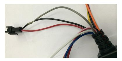
• Connect the SmartStart and the EVO-ONE together with the supplied cable. Or modify a Fortin DataLink cable as shown.
